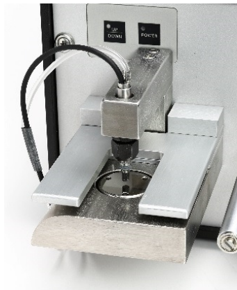
Contact Sensor Stand Manual Parallelism-Adjustable Anvil option for CX-1025a model. Allows manual parallelism adjustments for contact sensor. Recommended for use with full range of specified film thickness.
