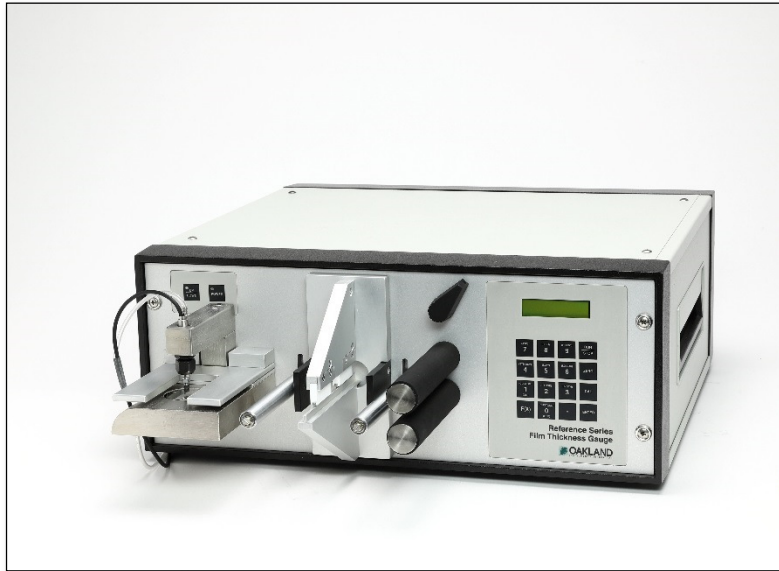
The Model CX-1025 AutoCal™ Film Thickness Gauge. Patent Rights Reserved
